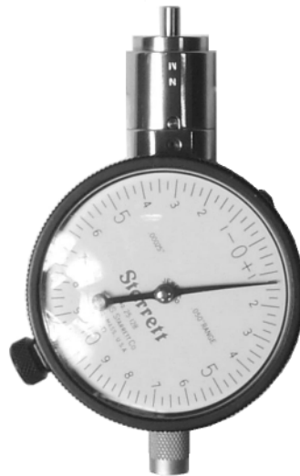
Figure D-6 Using the connector gage
